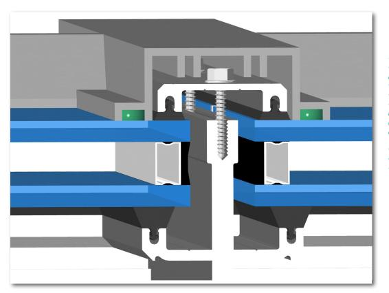
The patented design of Tremco's Spectrem (R) Restoration Overlay allows it to encapsulate leaking purlins while completely enclosing the silicone sealant bead. The result is a clean, aesthetically pleasing appearance plus an extra layer of protection that shields the sealant bead from exposure to the elements and eliminates air and moisture penetration.
